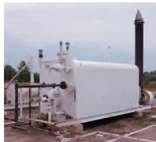
A heater-treater at one of the Marlow wells has the job of separating gas, water, and oil, which come out of the well mixed in a frothy emulsion. Under heat and pressure, the gas bubbles out of the mixture, while the denser water settles to the bottom.
