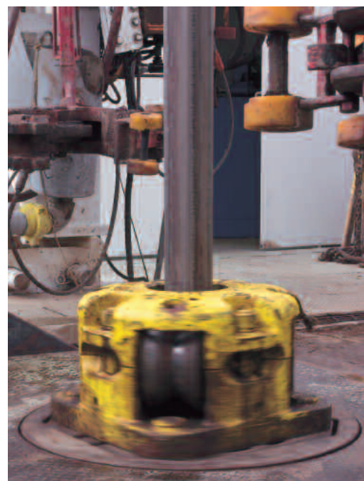
The main hoist on the Marlow rig ( above ) supports the drill string and regulates downward force. The black hose supplies drilling mud, which is pumped down the bore of the pipe. The rotary table ( below ) turns the drill string, transmitting twisting force to a special length of drill pipe called the kelly.
