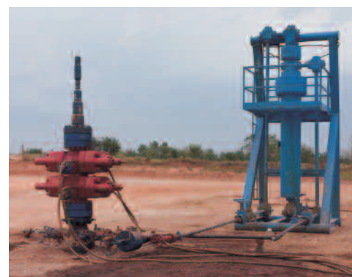
Another Chesapeake Energy well near Marlow had been drilled but was not yet in production when the photograph above was made. The wellhead, at left, still has a blowout preventer in case any high-pressure fluids are encountered. The apparatus at right is a sand separator, used to remove excess sand or “proppant” from the product stream. The proppant ( below ) consists of crush-resistant synthetic spherules that are forced down the well to prop open cracks in the oil- or gas-bearing rock layers.
