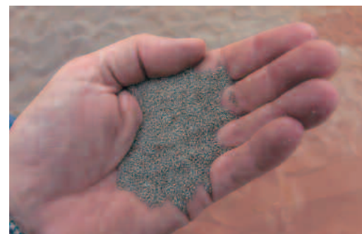
Another Chesapeake Energy well near Marlow had been drilled but was not yet in production when the photograph above was made. The wellhead, at left, still has a blowout preventer in case any high-pressure fluids are encountered. The apparatus at right is a sand separator, used to remove excess sand or “proppant” from the product stream. The proppant ( below ) consists of crush-resistant synthetic spherules that are forced down the well to prop open cracks in the oil- or gas-bearing rock layers.
