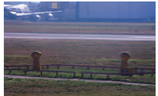
The twin pods staring at each other, above, measure runway visual range, or atmospheric clarity. Below is the most basic of all aviation weather instruments: the wind sock.
